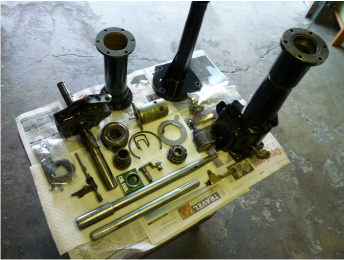
3. A disassembled Borg Warner that has been modified for a Model A. The original configuration is from a "modern" Ford car as it has the "long" housing.
