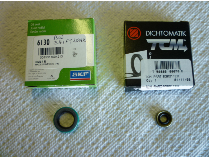
16. Two other seals are also important to control oil leakage. The one at left is inserted into the shift lever boss. The one at right is inserted into the solenoid shaft boss. Both seals are available from a bearing supply house. It is prudent to change both when overhauling a Borg Warner overdrive.
