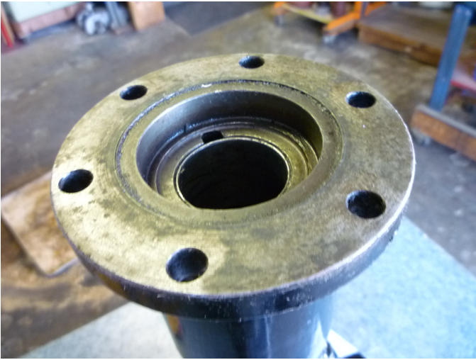
15. The output section of a Borg Warner overdrive modified for a Model A incorporates some type of an oil seal. This particular modification uses a large automotive seal that is inserted into the recess of the flange.
