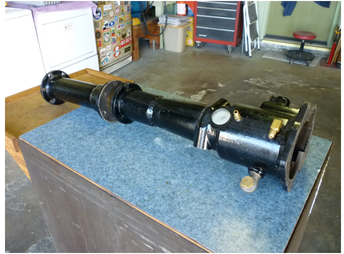
5. The aft section is also taken from the rear section of a Model A torque tube. A mating flange is welded to the aft end of the "long" Ford Borg Warner overdrive housing. When using the Studebaker or Nash overdrives a mating flange can be welded to the aft section of the Model A torque tube and mated directly to the aft end of the overdrive housing.
