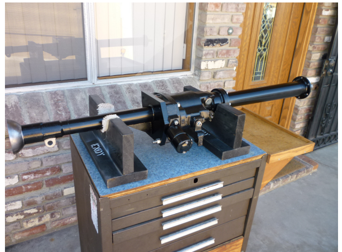
1. This Borg Warner Model A Modification was made from either a Studebaker or Nash with the short housing.
