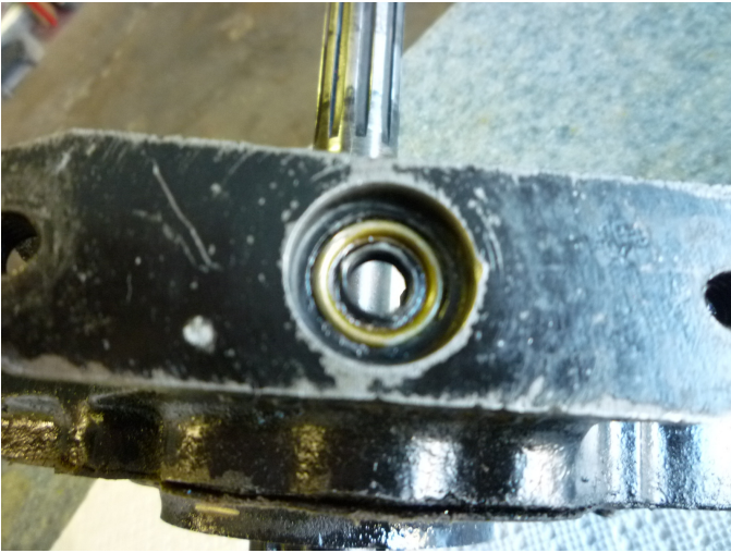
20. The solenoid boss is shown with a new seal installed.
