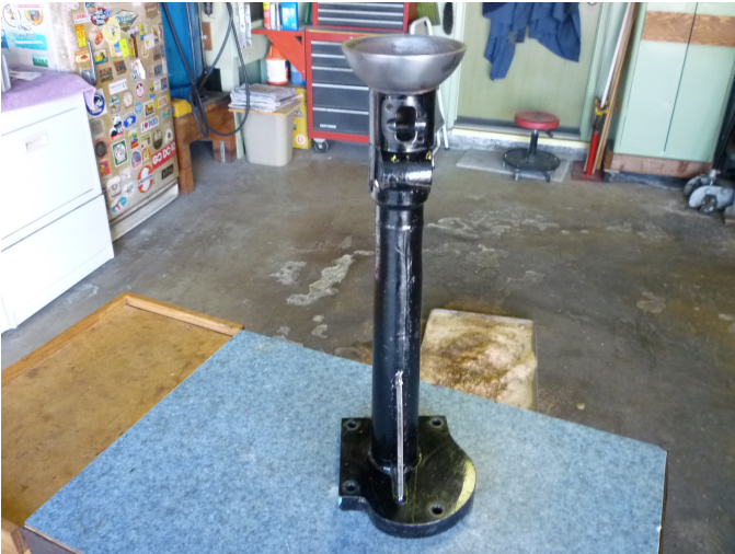
4. The front section is taken from a Model A torque tube and is sectioned and welded onto a mounting flange that mates to the front of the Borg Warner overdrive housing.
