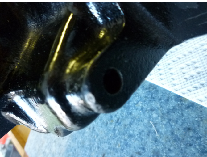
22. The hole shown in the housing is where the small plug is inserted after the inside shifting lever is rotated to engage the outside shifting lever during assembly.
