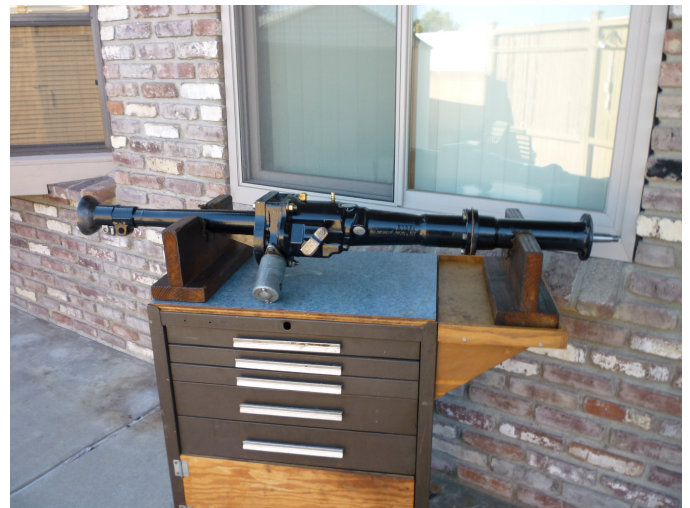
2. This Borg Warner Model A modification was made from a Ford with the long housing. The long housing modifications have a tendency to crack where the aft section is welded to a flange.
