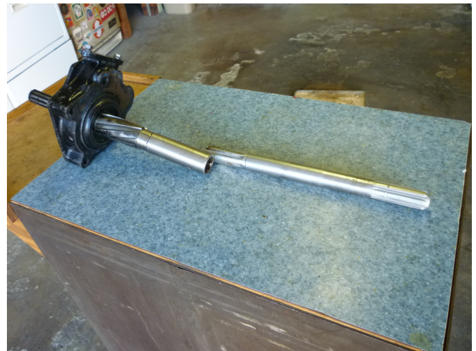
6. The input shaft (at right) is sectioned from a Model A drive shaft and a spline is machined onto the end that mates with a spline coupler that has been pinned and welded to the input shaft (at left) of the Borg Warner overdrive.
