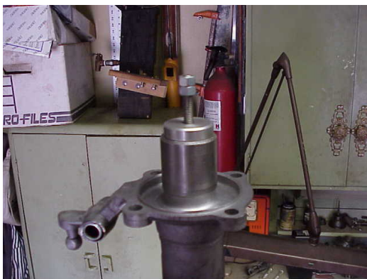
Carrier pre-load tool inserted
