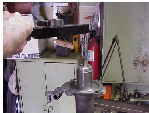
Measuring carrier pre-load
