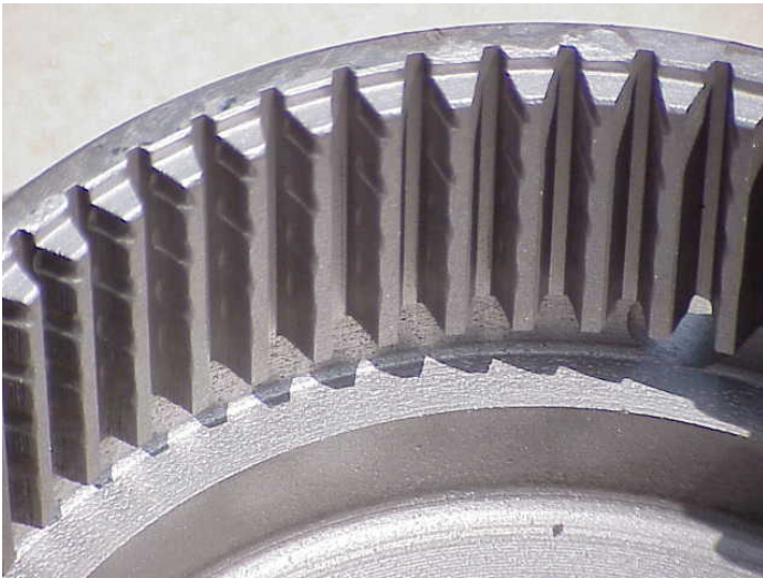
Notches worn in the flywheel
