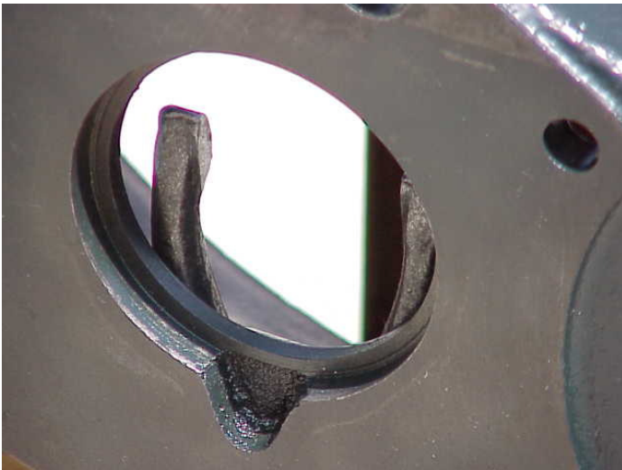
Oil baffle and snap ring mounts in recess
