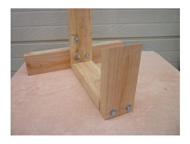
The 8" transmission support piece is attached to the rear of the base piece with two lags.
