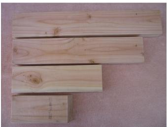
One ten-foot long 2X4 will make two stands with only a few inches of scrap left over. Four pieces for each work stand need to be cut to the following lengths. Top to bottom, 21", 18", 12", and 8". The 8" piece has one end cut at a 20 degree angle.
