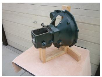
A transmission housing is shown attached to the bell housing. The work stand will easily support the weight of a bell housing and a fully assembled transmission.
