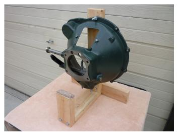
A piece of carpeting is attached to the top of the transmission support with staples and glue to prevent scratching a newly painted transmission housing. The 20-degree angle cut into the support will fit the bottom angle of the transmission housing.
