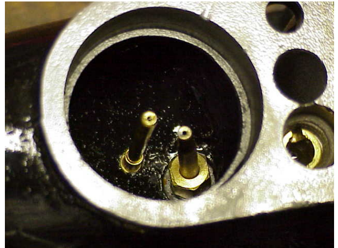
There should be no fuel leaks around either jet
