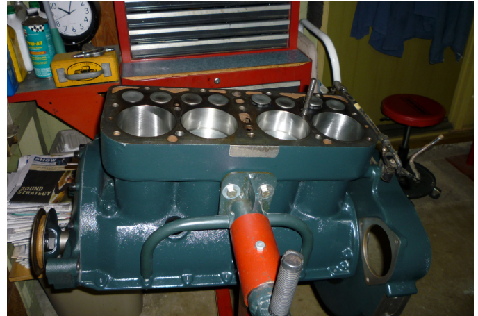
The #8 stud sits right next to the narrow area between #3 and #4 cylinder.
