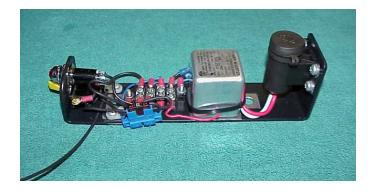
The complete assembly is shown above. The inverter is the square looking device in the center. The power outlet is to the right. The power outlet points straight down when installed under the dash rail. A single wire runs from the terminal strip to the negative 6-volt battery voltage. The power switch and the indicator lamp are to the left. The entire assembly is grounded by virtue of mounting it under the dash rail.
