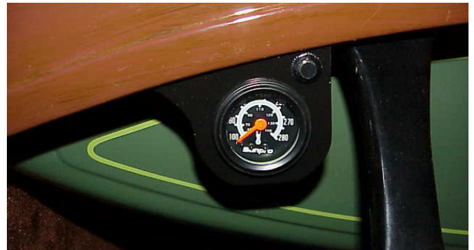
The little switch in the upper right corner of the bracket is a momentary push button switch wired to the ammeter that will give you a quick peek at the gauge while driving at night.
