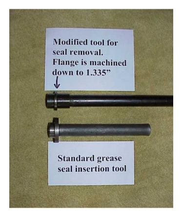
The tool in the top of the photo is a grease seal insertion tool with the flange turned down to 1.335" (arrow indicates flange) and it is attached to a five-foot length of  $\frac{1}{2}$ " water pipe. The tool in the bottom of the photo is a standard grease seal insertion tool attached to a short length of pipe used to install a grease seal into a torque tube.
