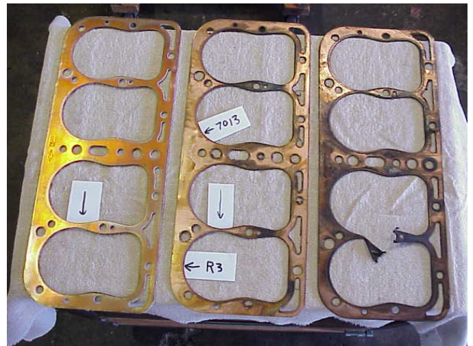
FelPro 7013 head gaskets. The gasket on the left is a -1, the arrow points to the area between #3 and #4 cylinders, note how wide the area is. The gasket in the center is a -3, note the area between #3 and #4 cylinders is very narrow. The number -3 is stamped on the gasket. The gasket on the right is a -3 that blew out between #3 and #4 cylinders.
